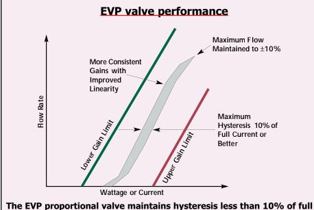
current over the entire flow range. More-consistent gains and linearity from valve to valve improve the performance of closed-loop control systems.
