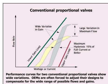
Clippard Instrument Laboratory has developed a new proportional valve, the EVP Series, that significantly reduces the variation in gain. It is based on the reliable and rugged design of the company's EV Series directional valve, which combines a simple design, low-power consumption, fast response, and long life—exceeding a billion cycles in some operations. The armature is the heart of the valve. It resembles a metal spider with flexing legs.
